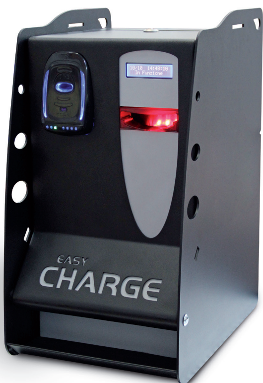
Version with Galaxy reading head and note validator
